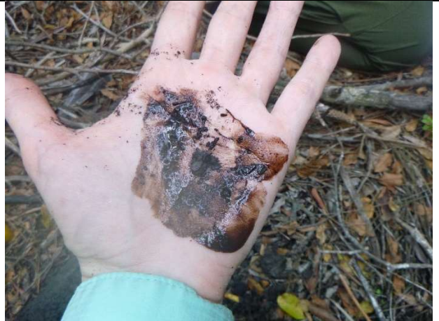
Photo 7: View of Ten Rub Fiber Test, showing less than 17% of fibers left.
